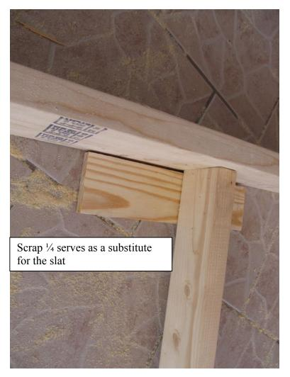
At this point the whole bed is upside-down. That was intentional. By doing this I can set the location for the center support by using some scrap wood underneath (the same thickness as a slat) to adjust the height properly. This made adding the support a breeze. No worries if it was in the right place, or if it was going to wander around (since it was pre-drilled). In hind-sight, maybe a couple extra screws toed in would have been a good idea. It couldn't hurt.
