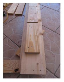
The slats are going to be supported on either side by the leftover 1x4's. These get screwed directly to the 2x6's, starting a couple inches from either end. This way there's clearance for the shorter 2x6's to make the outer box. Measure 3/4" from the edge, or use a scrap piece of wood to gauge where these 1x4's will sit. This way the top of the foundation is even from end to end. The old one was bumpy, as thei slats sat on top of the rails.
