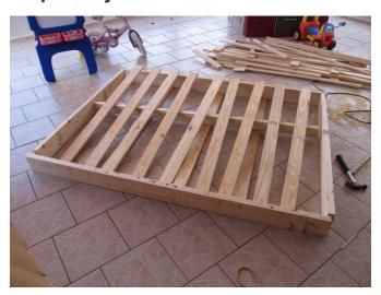
I described this a bit earlier, but perhaps the picture makes more sense. It's a box made from 2x6's on the outer perimeter. A 2x4 is laid length-wise in the center-line to prevent sagging in the middle. The "scrap" 1x4's will be used on the inside of the 2x6's for the slats to sit on. Of the 12 1x4's that were cut, 9 will go on top (for the mattress), and 3 will go on the bottom to prevent bowing out on the bottom).
