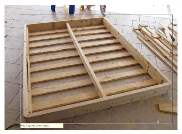
This part was a bit boring, but that's better than exciting (or frustrating). Flip the bed right-side-up. Because the 1x4's are so thin, and you're driving screws so close to the edge, predrilling is a necessity. I just used my countersink, as it penetrated deep enough with the "bit" part to prevent splitting by the screw, and the countersink kept the head from splitting the wood as well.
